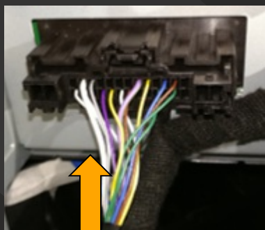
Connect to factory A/C cable
