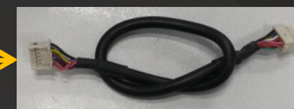
Knob line connect Mainframe with FRONT_COVER_ASM
