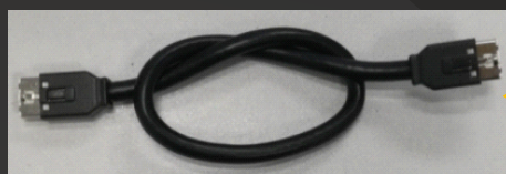
USB line connect Mainframe with FRONT_COVER_ASM
