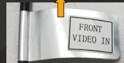
Marked FRONT VIDEO IN Line Connect to Front Camera (optional)
